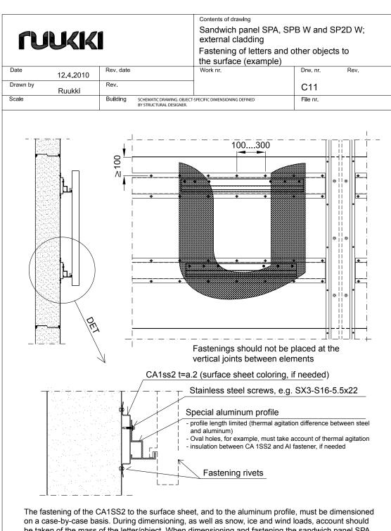
be taken of the mass of the letter/object. When dimensioning and fastening the sandwich panel SPA element, account must be taken of any additional loads caused by objects to be attached.
